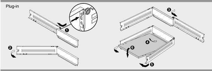
Drawer Front Assembly and Removal - Standard Bracket
