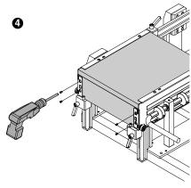
Secure back panel using screws.
