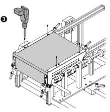
Secure bottom panel using screws.
