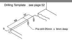
Cutting Dimensions for 16mm Chipboard
