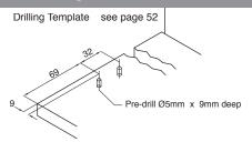
Cutting Dimensions for 16mm Chipboard
