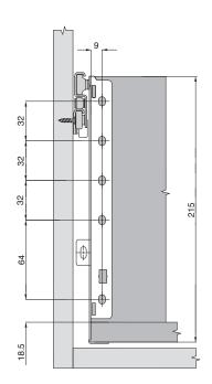
Cutting Dimensions for 16mm Chipboard
