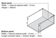
Pre-drilling Dimensions of Bottom Panel for Plug-in
