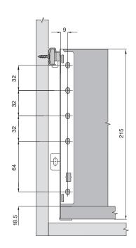
Cutting Dimensions for 16mm Chipboard
