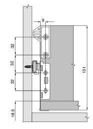
Cutting Dimensions for 16mm Chipboard
