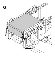
Insert back and bottom panels. Slide in drawer sides. Activate locking clamps to hold drawer together.
