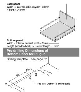
**DIN A4 Along Drawer Width DIN A4 Along Drawer Length** K 329mm Cross Hanging Rail Cutting Cross Hanging Rail Cutting Width = Internal cabinet width - 44mm Width = Internal cabinet width -44mm 329mm BOA Internal cabinet width = 362mm Min. drawer length = 450mm 705
