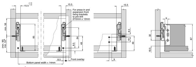
() Inner Drawer \*Add 8mm when used with 201.000 Drawer Front Locking Piece.
