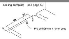
**Cutting Dimensions for 16mm Chipboard**
